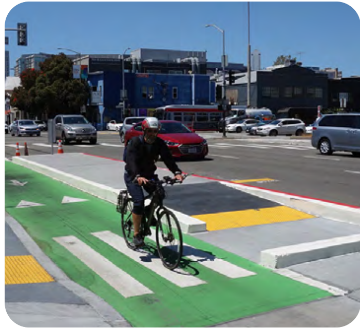
① Class IV More extensive- Painted and physical elements separating cyclists
