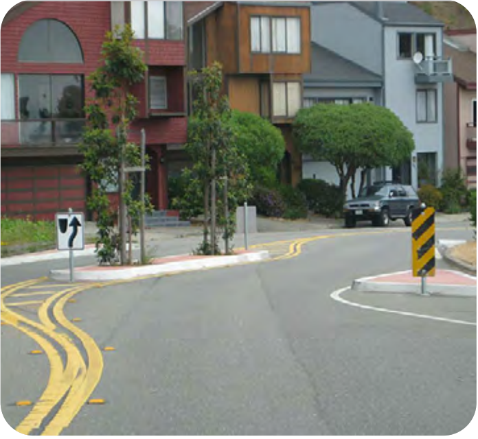
⑨ Chicanes and Pinch-points- Slow traffic on local streets while providing more space for amenities.
