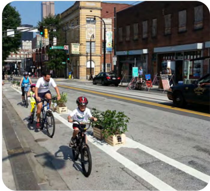
② Class IV Less Intense- Separated bike lanes using simple buffer and vertical separation
